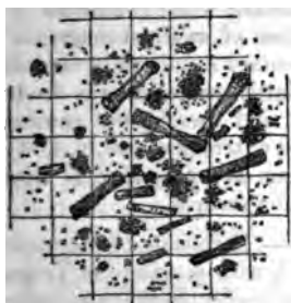
Microscopic Appearance of Light Carbonate of Magnesia.
